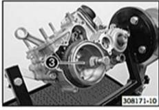
Mount special tool 3, apply counterpressure, and pull off the rotor by screwing in the screw.
